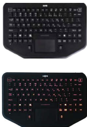
One touch button illuminates red monochrome backlight
